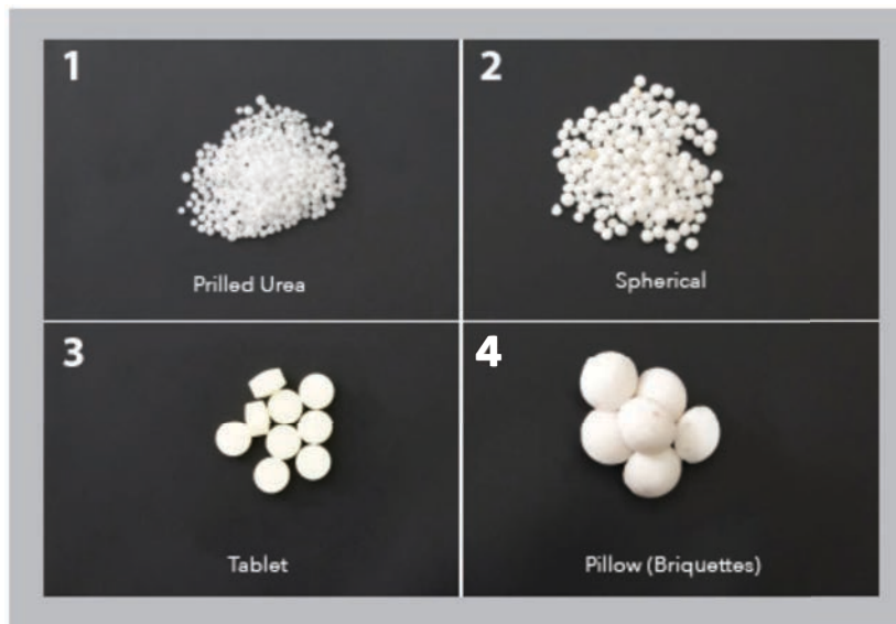
Figure 3. Prilled Urea and Urea Briquettes of Various Shapes
