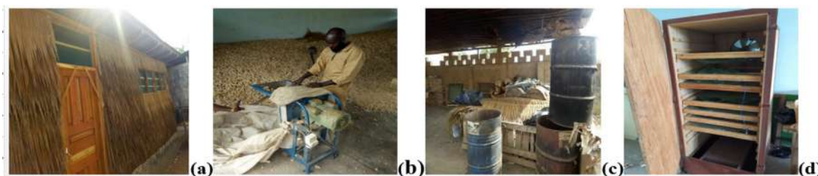
Board 3 : (a) Cultivation shelters built in straw; (b) Corn cobs crushing; (c) Home-made pasteurizer; (d) Handcrafted electric gas dryer with fan
